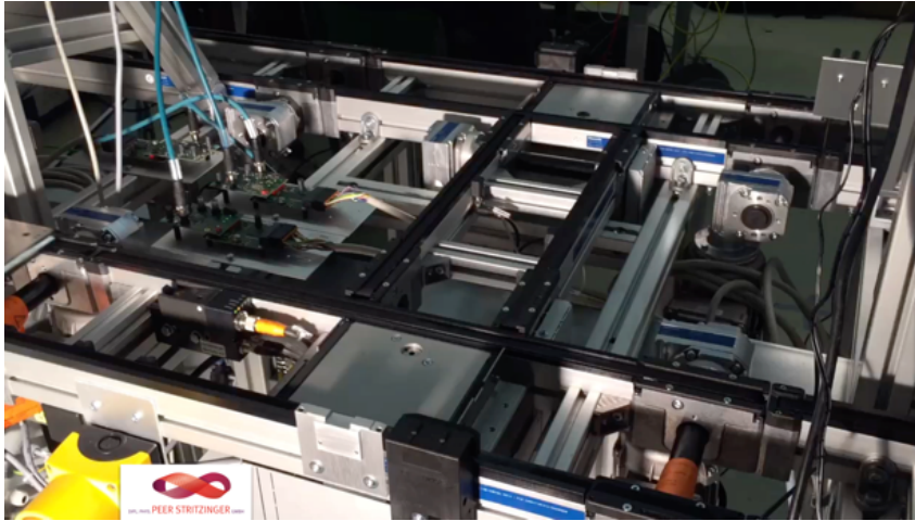
Figure 2.4.2: RFID Reader Prototype Boards controlling a conveyer belt distributedly
