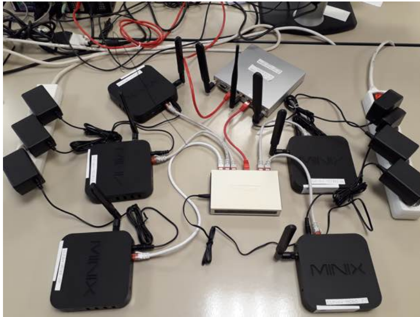
Figure 2.2.3: A group of five MINIX NEO Z83-4 devices forming a cluster.
